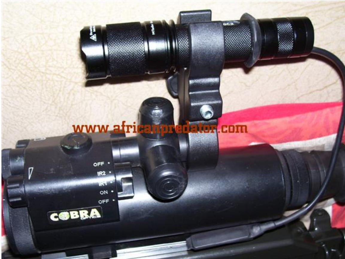
This shows the Infra red light fitted above my rifle night vision scope, this shows the light without a funnel to stop side leakage, below is a picture with a funnel fitted. The pressure switch is really handy for putting the torch on **quickly and quietly!**
